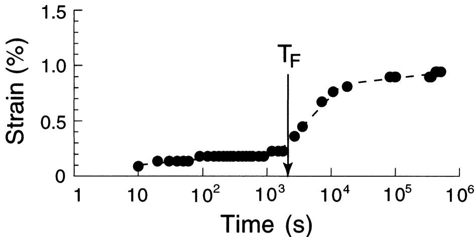
Figure 5.—Creep curve for sample loaded to 20% of yield stress (Fig. 1), re-scaled on a logarithmic time axis so that the initial stages of creep are emphasised.  $T_F$  is the approximate duration of conventional tensile tests performed on spider dragline at a constant strain rate of  $10^{-4} \text{ s}^{-1}$ ; such tests are typically completed (the fiber fails by breaking) in less time than it takes for creep to make its most significant contribution.
