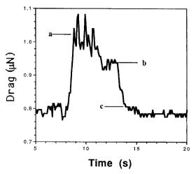
Figure 13.—Drag generated on the surfaces of a theridiid hatchling (0.18 mg). The horizontal lines indicate drag at different postures: (a) all legs extended and waving; (b) all legs loosely held against the body; (c) all legs tightly held against the body. Note that a very small change in posture (from b to c) resulted in a substantial reduction in drag.
