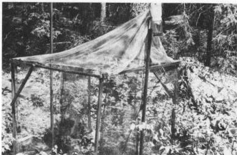
Fig. 1.—Modified Malaise trap for capturing insects and spiders in spruce-fir forests, west-central Maine.
